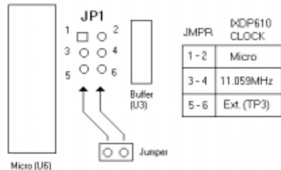
**Figure 5: Placement of Jumper for IXDP610 Clock Selection**
