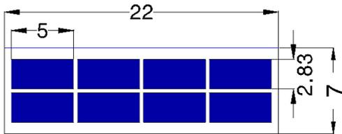
**Front-side View details**
